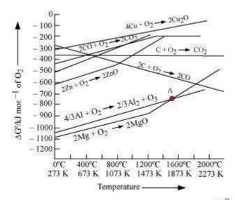
The above figure is a plot of Gibbs energy  $(^{\Delta G^{\Theta}})$ vs. T for formation of some oxides. It can be observed from the above graph that a metal can reduce the oxide of other metals, if the standard free energy of formation  $(^{\Delta f}G^{\Theta})$ of the oxide of the former is more negative than the latter. For example, since  $^{\Delta f}G^{\Theta}_{(Al,Al_2,O_3)}$  is more negative than
