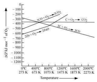
Reduction of ZnO to Zn is usually carried out at 1673 K. From the above figure, it can be observed that above 1073 K, the Gibbs free energy of formation of CO from C and above 1273 K, the Gibbs free energy of formation of  $CO_2$  from C is lesser than the Gibbs free energy of formation of ZnO. Therefore, C can easily reduce ZnO to Zn.
