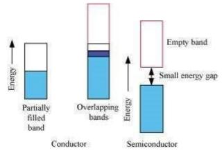
On the other hand, the valence band of a semiconductor is filled and there is a small gap between the valence band and the next higher conduction band. Therefore, some electrons can jump from the valence band to the conduction band and conduct electricity.
