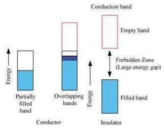
On the other hand, in the case of an insulator, the valence band is fully- filled and there is a large gap between the valence band and the conduction band.
